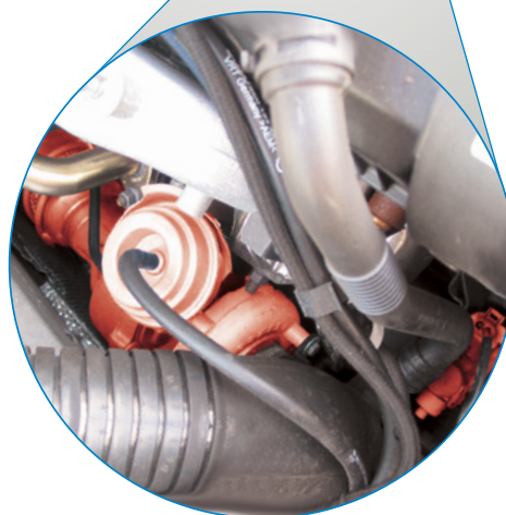
Pressure transducer and VTG charger (highlighted in red) in the Audi A4 TDI
